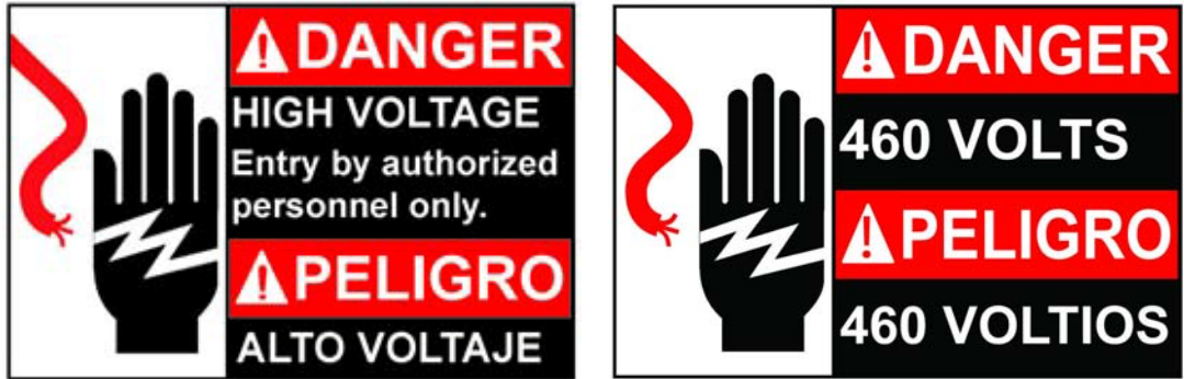
Figure 2-1 - Red & Black labels indicate DANGER hazards
